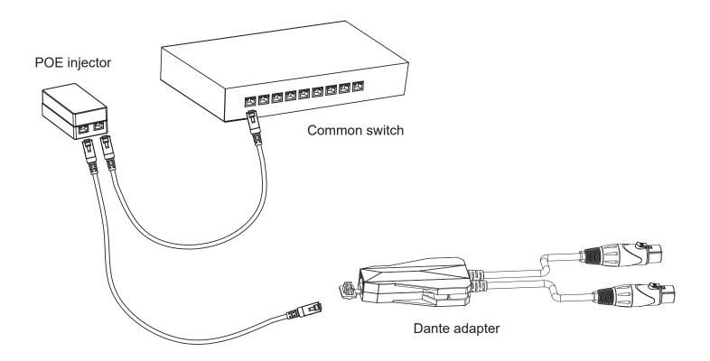
3. Ensure LED is solid on the RJ45 port of Dante adapter (Blinking yellow, solid Green)
