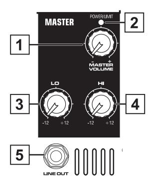
**D1** - MASTER volume control fader. From minimum to maximum (clockwise). This fader affects the
