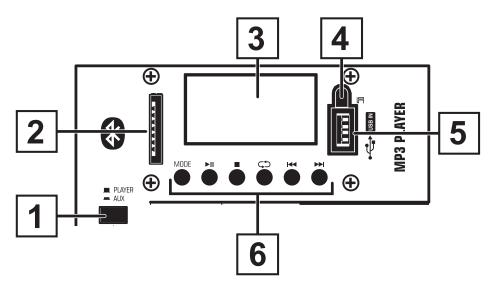
**B1** - Channel 1 input selector. Allows you to decide if the player or the Aux input will be active on channel 1 of the mixer.
